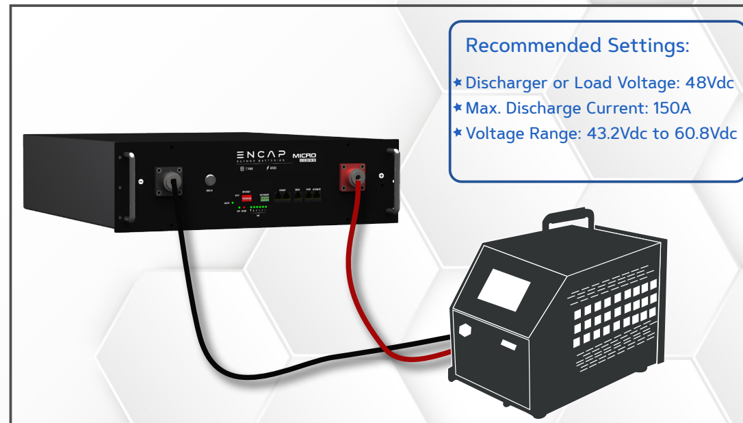
Figure 12: Discharging Module from discharger
