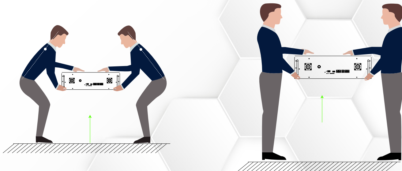
Figure 4: Lifting up the Module
