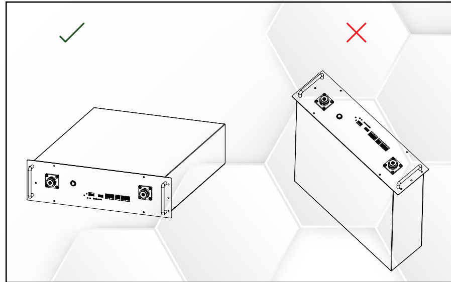
Figure 7: 1) Correct angle position 2) Wrong angle position
